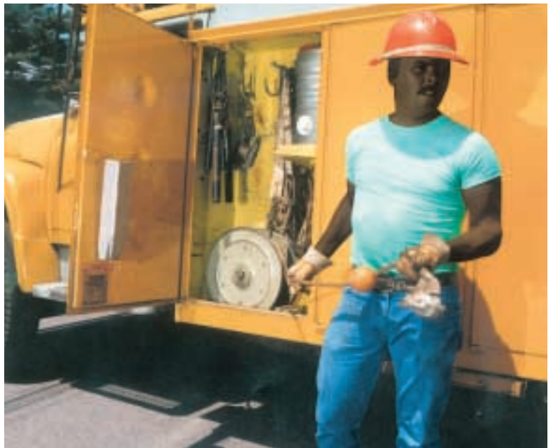
A truck-mounted Hannay reel handles grounding cable for mobile utility applications.
